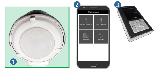
1) The Wattstopper FSP sensor. 2) The phone app interface for the Z321B. 3) The FSIR-100 wireless configuration tool for Z221B.
