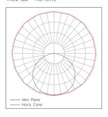
Relative Luminous Intensity RCL G2 - with Frosted Diffuser
